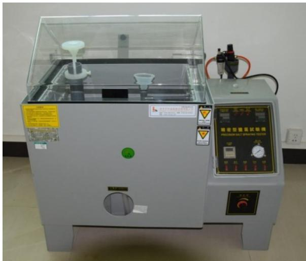
**Salt mist tester to test components, electronic element, metal and etc corrosion**
